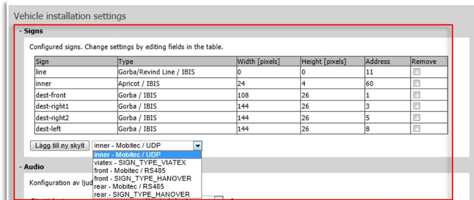
The first column in the list contains “Sign names”, determining the information presented on the sign. If the sign name is “front”, for instance, the content and layout will be adapted for presentation on the front sign of the bus. For internal signs/displays, there are many custom layouts so there are several alternatives for these. The table below describes various sign names in use by our customers.
