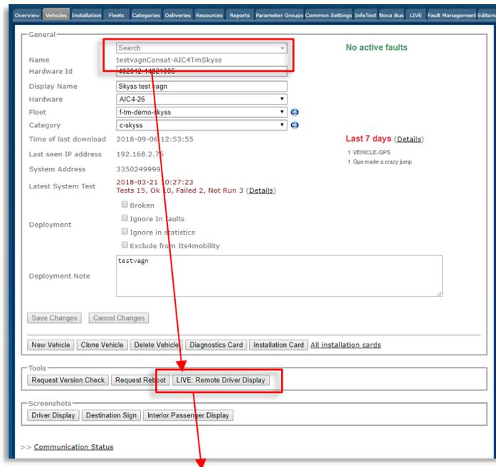
3. **The LIVE view tab is opened**, showing the driver interface (it may take a few seconds to load), and below, the current internal display (if available) and a map with a vehicle trail showing the latest vehicle positions - reported during the past 10 minutes (configurable time).
