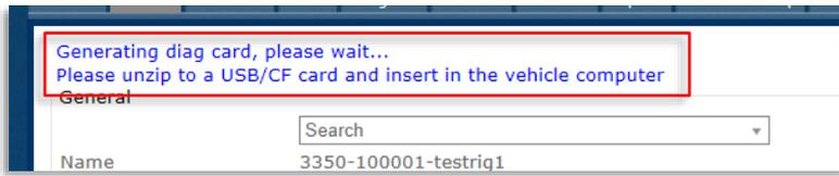
4. As stated in the message, when the generation has finished, unzip the file to the USB stick/Flash card (CF or SD depending on the computer).
