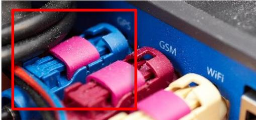
3. Run the GPS System test. If OK (GPS connection), Proceed with the test in step 4. Not OK: Change antenna.
